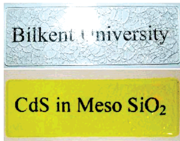
Figure 4. Photographs of the monoliths prepared on a glass slide indicating the samples are transparent before (top) and after (bottom) \text{H}_2\text{S} treatment.
